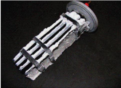
**Figure 4 Scale deposits on a cell**
